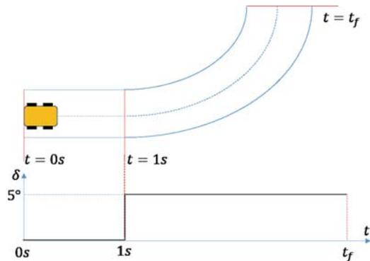
Fig. 2 The step input of front steering angle
