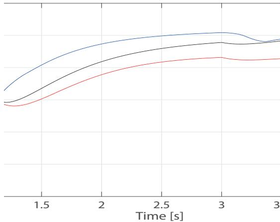
Fig. 3 Time response of  $d(t)$ . In the whole simulation time, the value of  $d(t)$  of the proposed method is smaller than that of the case without control. And the value of  $d(t)$  of the proposed method is smaller than that of the conventional method since 1.05s
