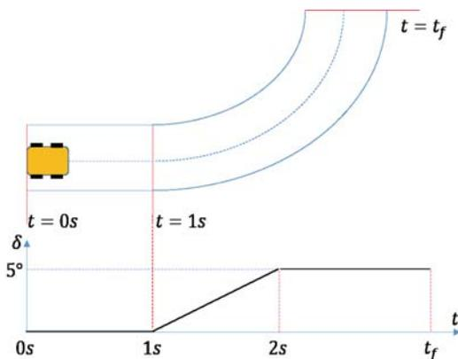
Fig. 4 The ramp input of front steering angle
