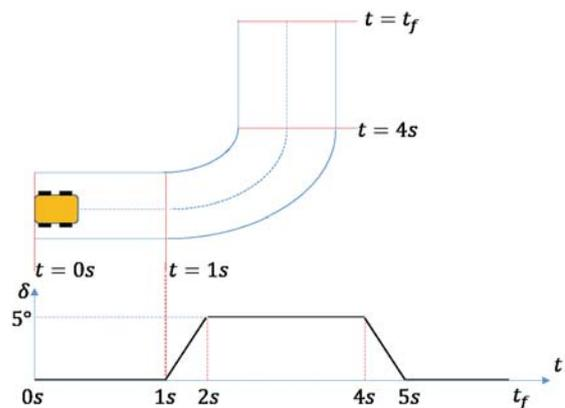
Fig. 6 The ramp input of front steering angle
