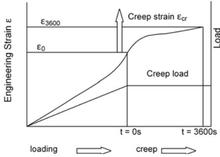
Fig. 1 Schematic illustration of the loading process
