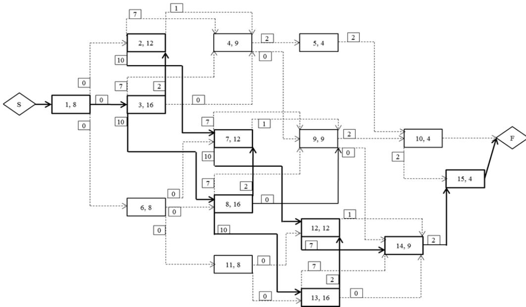
Fig. 11 PDM schedule network of laying cement slabs
