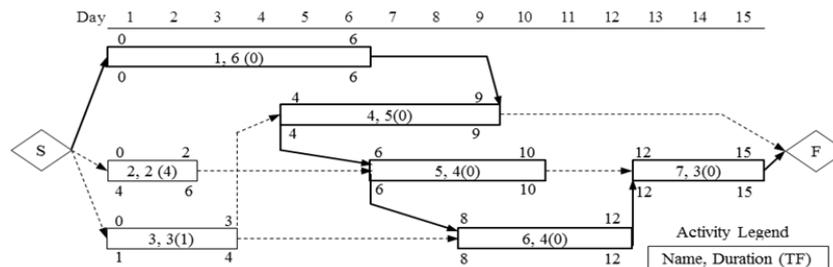
Fig. 3 PDM schedule network on horizontal time scale
