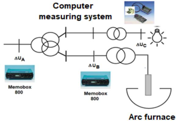
Fig. 3 Places of measurement of electricity quality parameters
