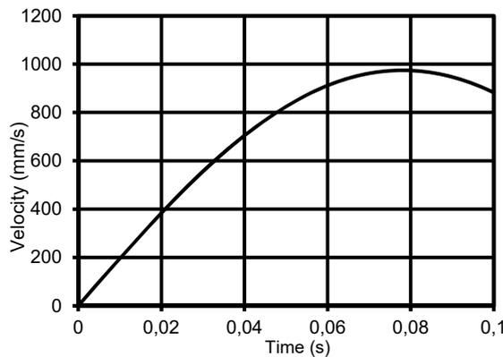
Fig. 5 Velocity of the mould base
