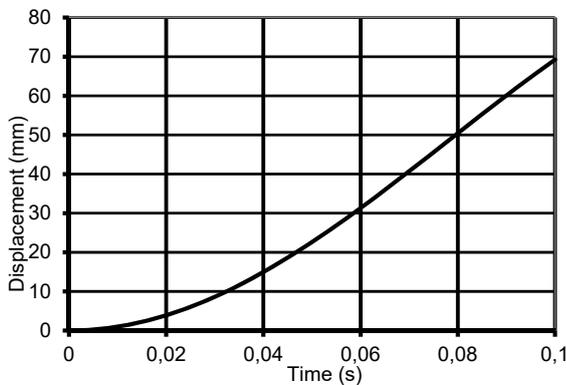
Fig. 4 Displacement of the mould base
