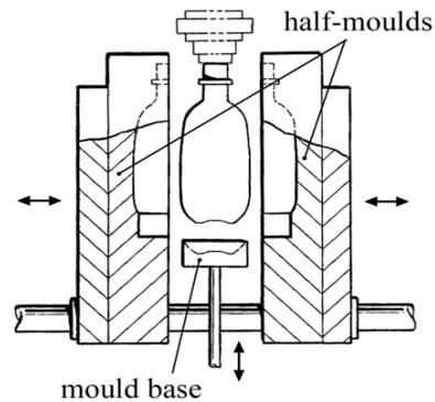
Fig. 1 The half-moulds and the mould base displacements in the typical blow-molding machines
