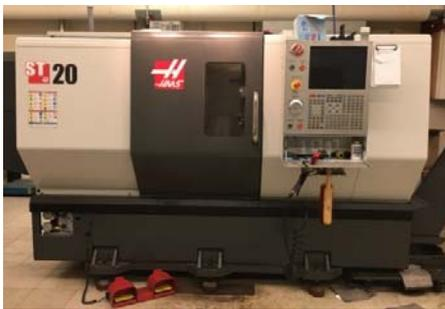
Fig. 2 HAAS ST-20 CNC Machine
