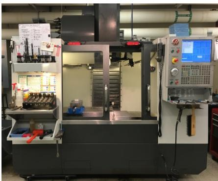
Fig. 3 HAASVF-2 TR CNC Machine
