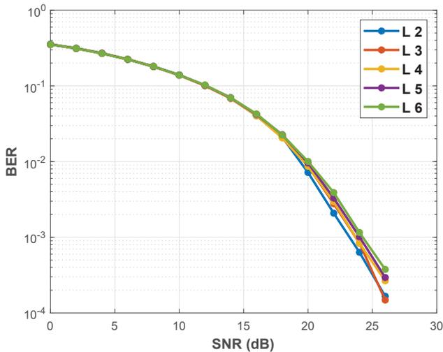
Fig. 9 BER for different channel length  $L$  with FFT size  $N = 512$  and  $QAM = 64$
