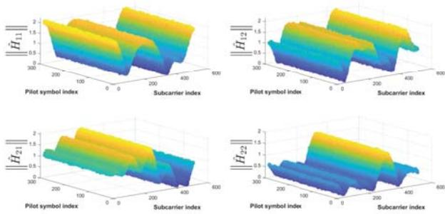
Fig. 4 Evolution of the estimated channel frequency response over all pilot symbols for all channels
