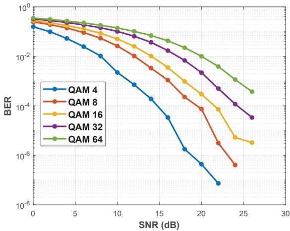
Fig. 8 BER for different QAM size with FFT size  $N = 512$  and channel length  $L = 6$
