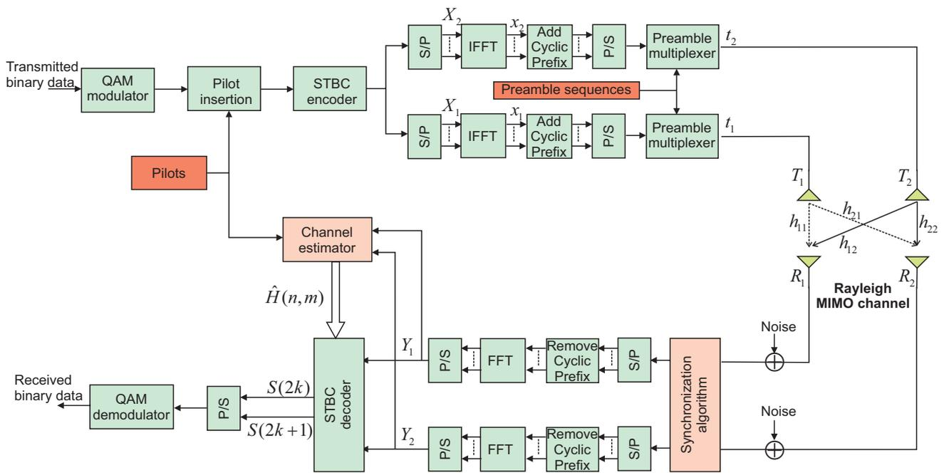
Fig. 2 Simplified block diagram of MIMO-OFDM system
