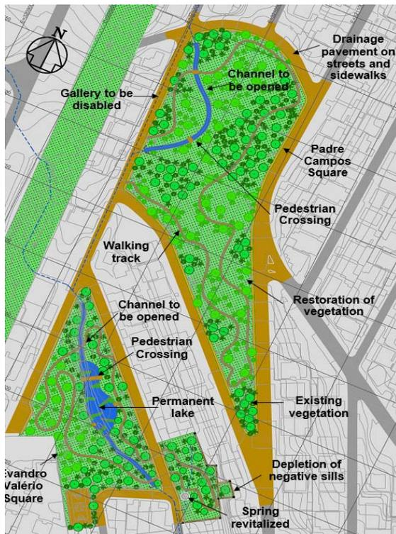
Fig. 9 Proposal of revitalization of the area - Plant of implantation.
