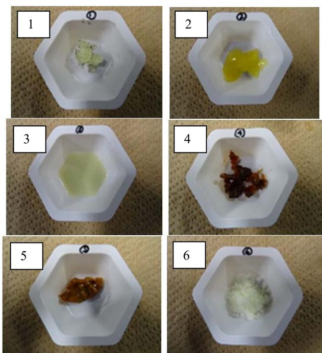
Fig. 7 Appearances of the solids after gamma-ray irradiation
