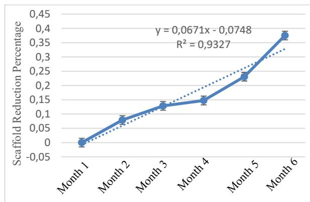
Fig. 3 The PCL scaffold degradation test charts, for six months, the rate of increase in weight loss percentage = 0.07 / month
