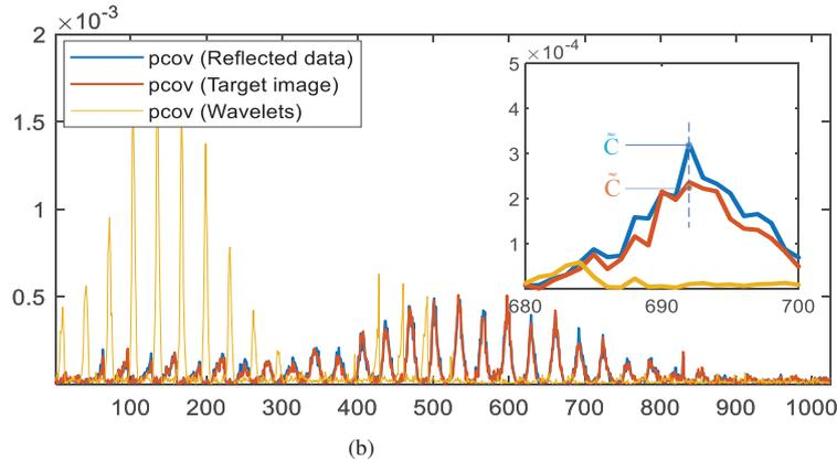
Fig. 5 (a) Sample sets of both reflected data and target image at the same location is built, for the calculation of augment covariance matrix related to that location. (b)  $\tilde{C}$  in the partial enlarged drawing are computed based on the sample sets given above, and the rest pseudo covariances are calculated in the same manner; and the resultant plots consist of pseudo covariances of the reflected data, the target image, and the wavelets coefficients, each of which has 1024 elements
