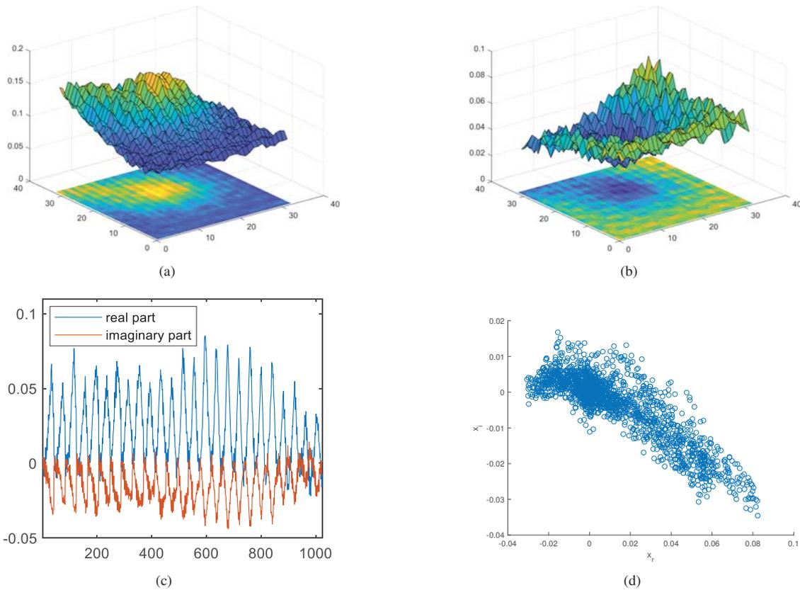
Fig. 3 Reflected data of a single-frequency measurement (19.26 GHz) is collected in a 2-D matrix, dimension of which is  $32 \times 32$ . (a) The real parts. (b) The imaginary parts. (c) The reflected data is reshaped as a  $1024 \times 1$  vector, the real and imaginary parts of which are plotted side-by-side. (d) Scatter plot of the 1024 complex-valued data, with " $x_r$ " being the real axis and " $x_i$ " being the imaginary axis
