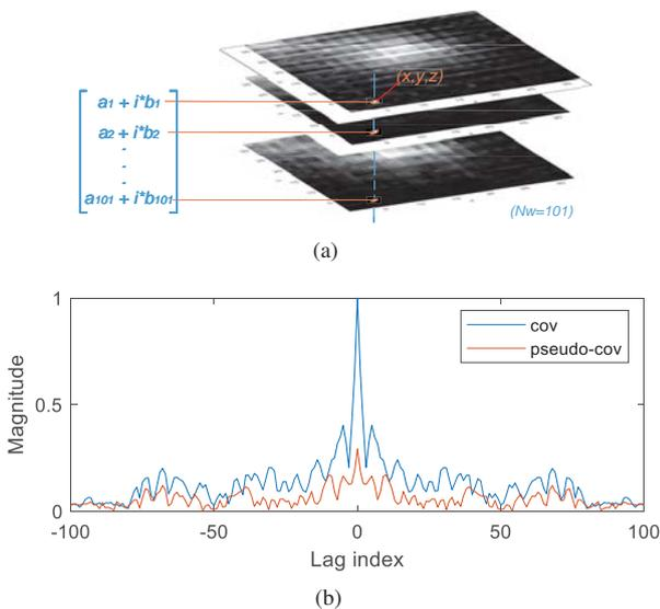
Fig. 4 (a) The multi-frequencies reflected data set is consist of data collected with  $N_\omega = 101$  different scanning frequency, ranging from 18 GHz to 26.4 GHz; And the complex scalar at location  $(x,y,z)$  is extracted from each frequency layer, to build a sample set for the particular location. (b) The covariance function and the pseudo covariance function is calculated based on the sample set  $\{a_1 + ib_1, a_2 + ib_2, \dots, a_{101} + ib_{101}\}$
