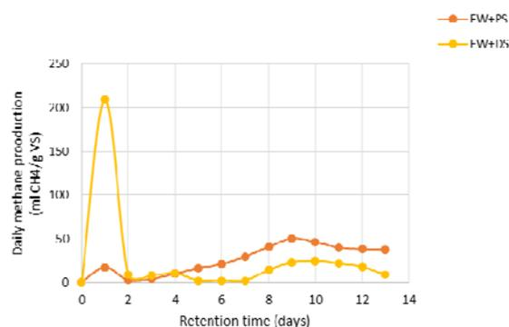
Fig. 3 Daily CH<sub>4</sub> production with two types of inoculum
