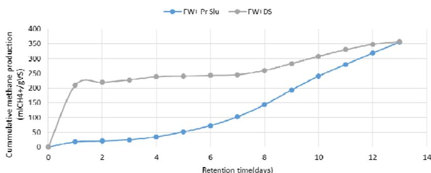
Fig. 2 Cumulative CH<sub>4</sub> production of FW with primary and digested sludge as an inoculum
