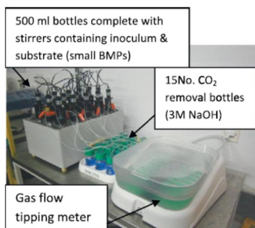
Fig. 1 Automatic CH<sub>4</sub> potential test system (AMPTSII)[19]
