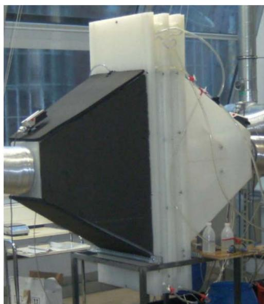
Fig. 4 Assembly of the absorber with air diffusers
