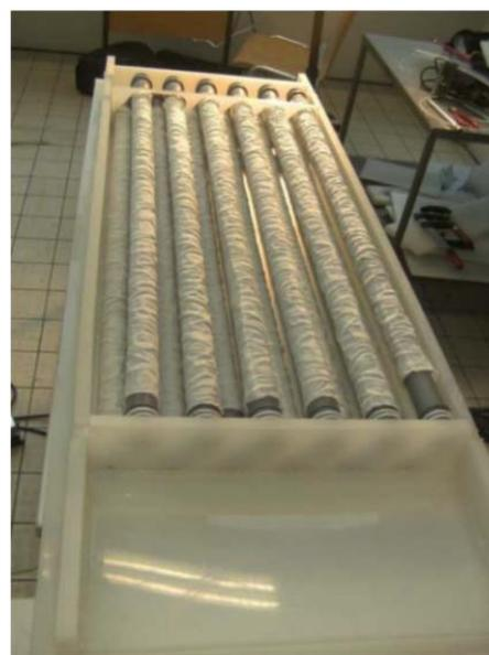
Fig. 3 PP tubes covered with textile sleeves
