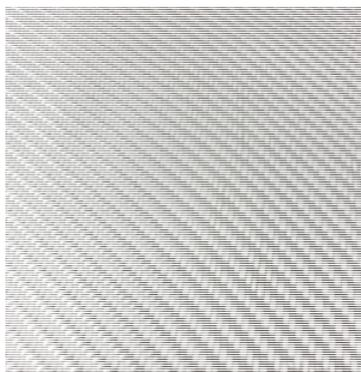
Fig. 1 Bidirectional fiberglass
