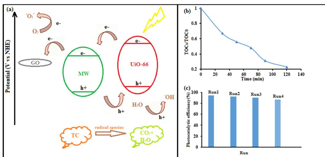
Fig. 5 The possible mechanism of photodegradation by synthesized photocatalyst under visible light irradiation (a), mineralization of TC in the photocatalytic process as a function of contact time (b); photocatalytic efficiency over four consecutive cycles (c)
