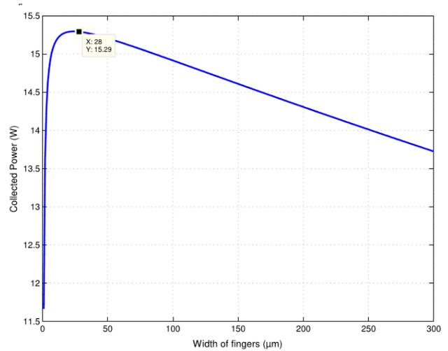
Fig. 4 Collected power according to width of fingers
