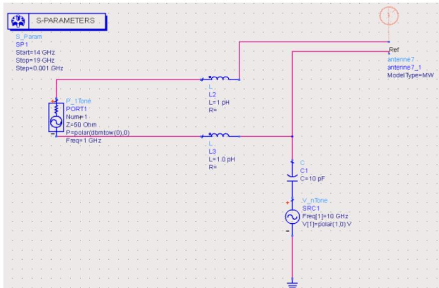
Fig. 7 Solar cell antenna decoupling RF/DC circuit
