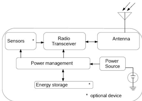
Fig. 2 Conventional wireless system block diagram
