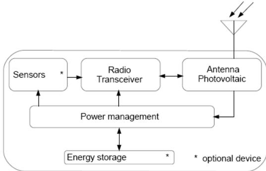
Fig. 1 Autonomous wireless system using the photovoltaic antenna
