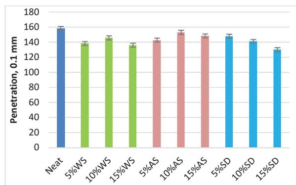
Fig. 4 Penetration values of pure and modified binders
