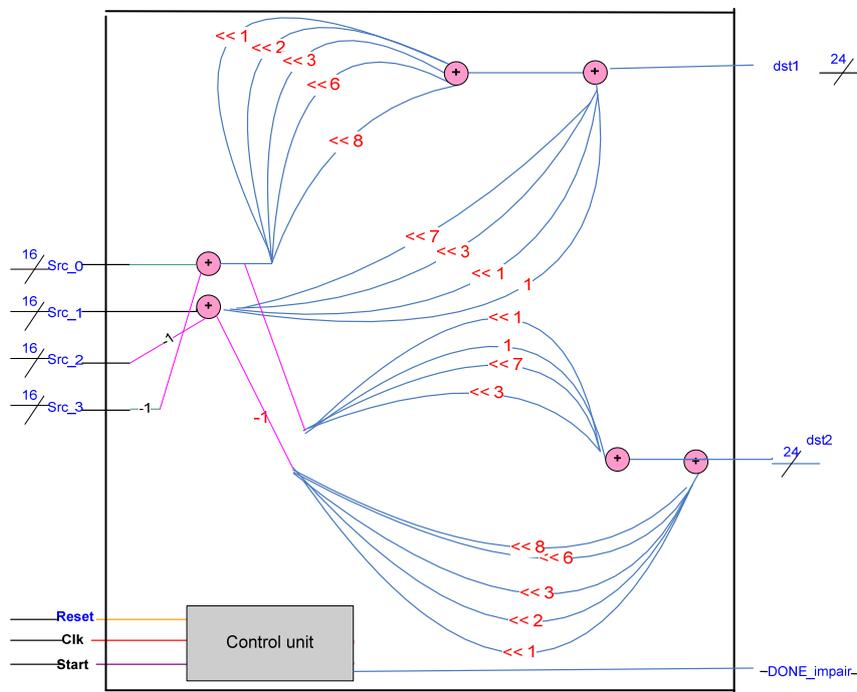
Fig. 6 The peer part of ICT\_4\_1D architecture: Bloc\_DCT4\_peer
