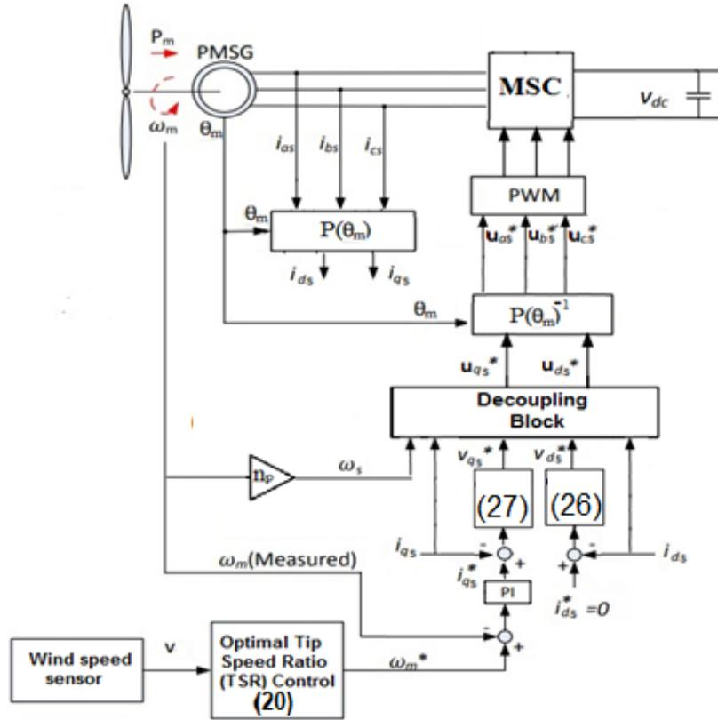
Fig. 5 Control block diagram of the MSC [9], [11]
