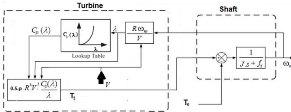
Fig. 4 Wind Turbine and Shaft Models [11]
