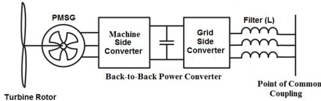
Fig. 1 WECS based on PMSG
