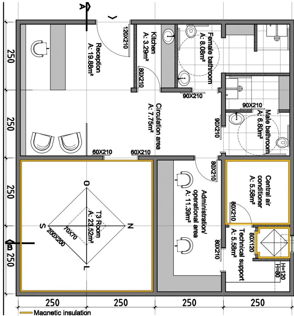
Fig. 8 Floor plan with the minimum configuration expected for the installation of the Device
