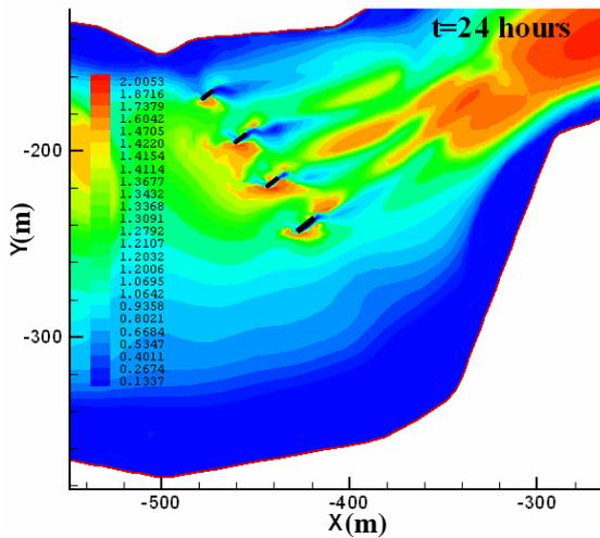
Fig. 7 Flow velocity field around the bridge piers for  $Q=914.63$  m<sup>3</sup>/s.
