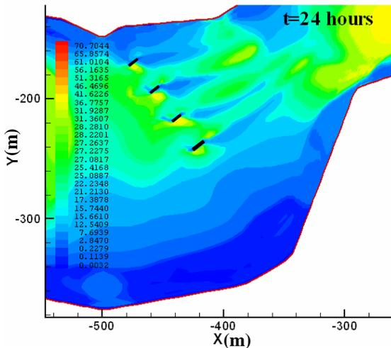
Fig. 8 Shear stress field around the bridge piers for  $Q=914.63$  m<sup>3</sup>/s.
