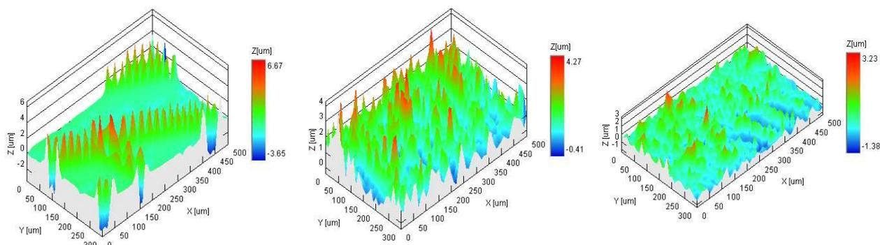
Fig. 4 The measured 3D profiles of studied samples of PS-TM, PS-ASM and PS-ESM (T = 10 min and I = 60 mA)
