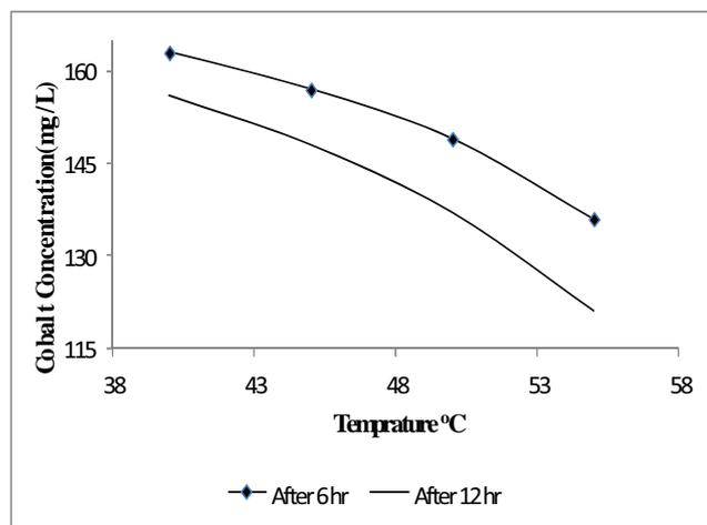
Fig. 2 Relative concentration of Co<sup>2+</sup> with temperature and time
