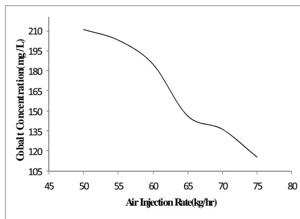
Fig. 3 Relative concentration of cobalt with air rate
