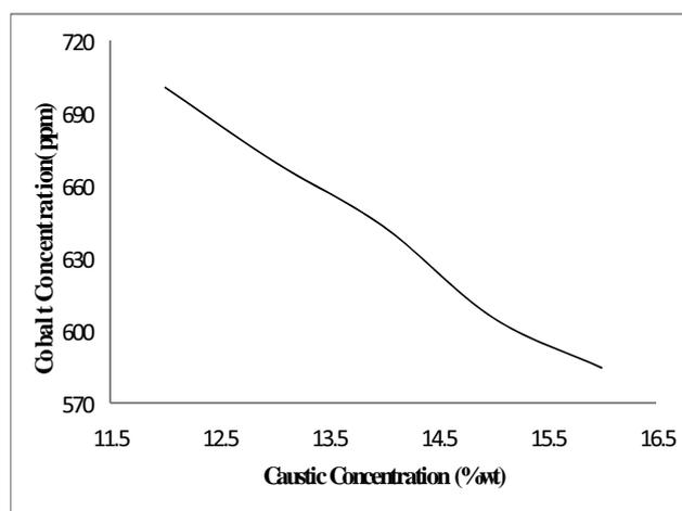
Fig. 1 Relative activity of  $Co^{2+}$  with caustic concentration
