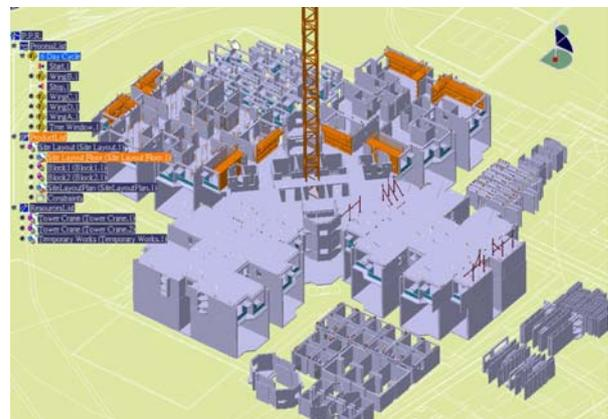
Fig. 1 Building block layout in virtual prototyping environment
