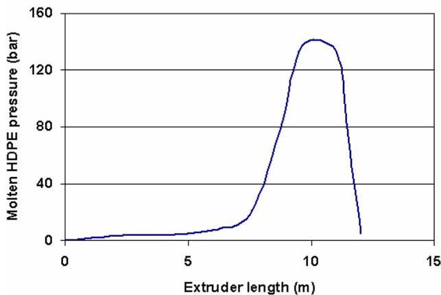
Fig. 2 Pressure profile in twin-screw extruders' length
