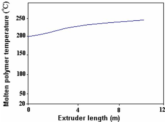
Fig. 1 Temperature profile in twin-screw extruders' length
