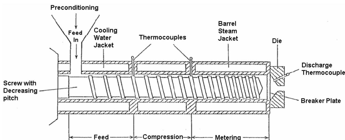
Fig. 1 Single-screw extruder
