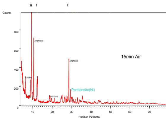
Fig. 7 Micro-waved & floated sample (air froth)
