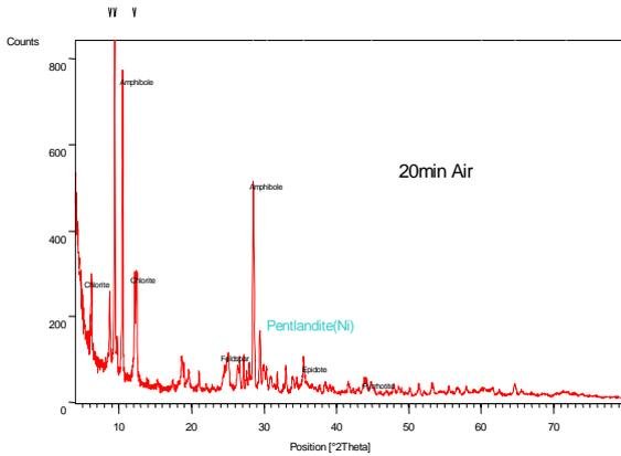
Fig. 9 Micro-waved & floated sample (air froth)
