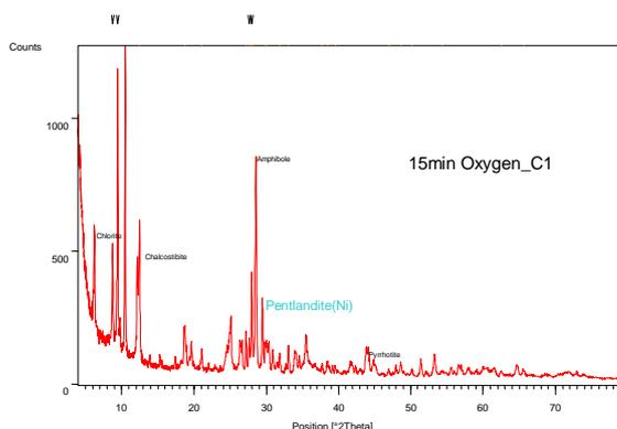
Fig. 8 Micro-waved & floated sample (Oxygen froth)
