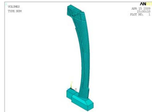
Fig. 3 Finite element mesh of the cable tower
