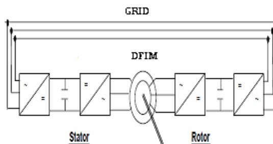
Fig .1 DFIM supplied by two PWM inverters
