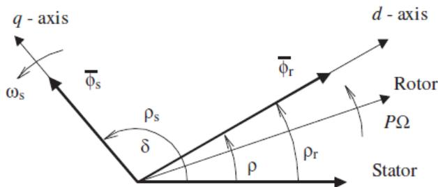
Fig. 6 DFIM vectorial diagram after orientation
