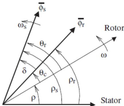
Fig. 5 DFIM flux relative armature position
