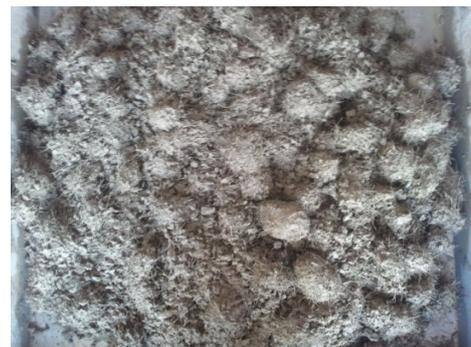
Fig. 4 Fiber ball Phenomenon (S44F1.25, S44V1.5, S51V1.5)
