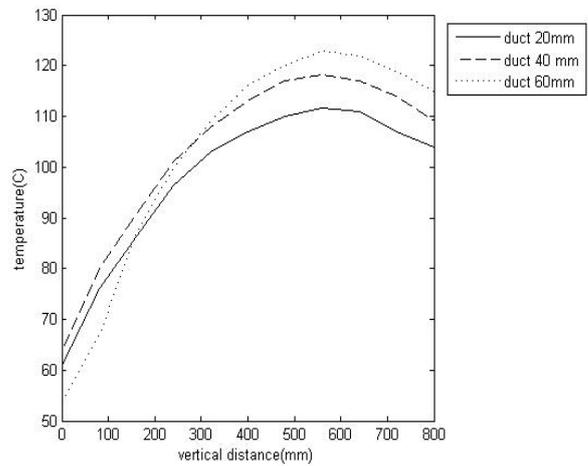
Fig. 8 Variation of temperature of outer surface at different air duct
