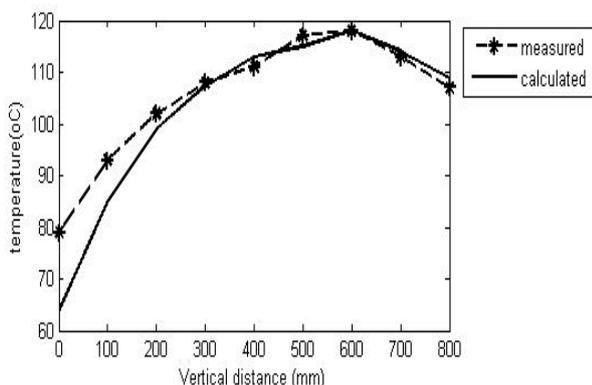
Fig. 4 Comparison measured and calculated temperatures at outer surface
