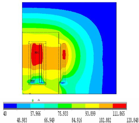
Fig. 5c Calculated temperature distribution at ambient 40°C
