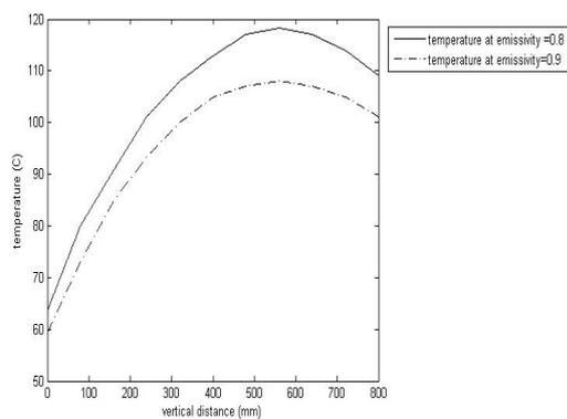
Fig. 10 Distribution of temperature at different emissivities
