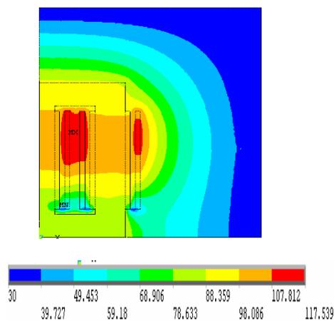
Fig. 5b Calculated temperature distribution at ambient 30°C
