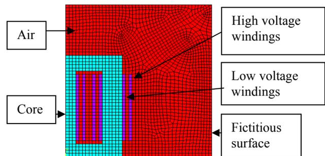
Fig. 2 Schematic of transformer with elements
