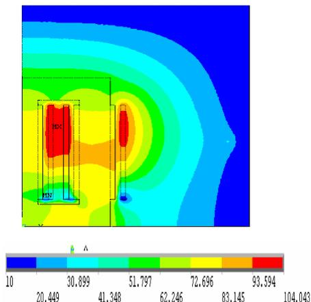
Fig. 5a Calculated temperature distribution at ambient 10°C
