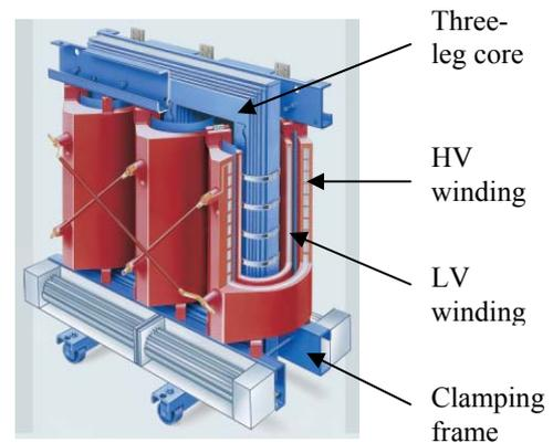
Fig. 1 Schematic view of cast resin transformer
