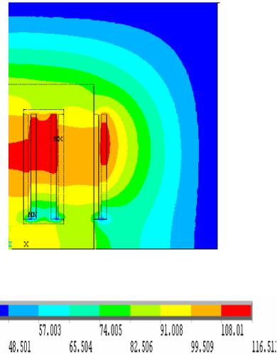
Fig. 7c Calculated temperature at air duct 20mm
