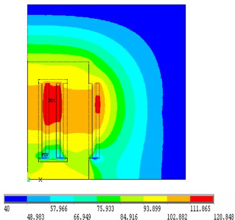
Fig. 3 Calculated temperature distribution at full load 800 kVA
