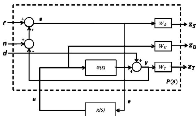
Fig. 4 General configurations for  $H_\infty$  control problems
