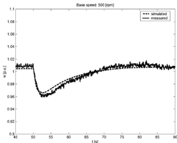
Fig 6 Speed of the turbine with PID controller
