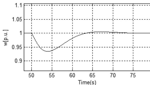
Fig 8 Speed of the turbine with  $H_{\infty}$  controller
