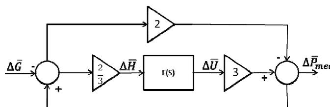
Fig. 3. Block diagram of the linear of turbine
