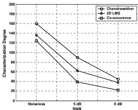
Fig. 4 Characterization degree of the Chandrasekhar filter coefficients, the 2-D LMS filter ones and the co-occurrence method features for various SNR values (Filter order of 3x3).
