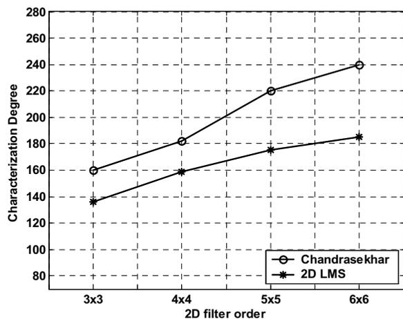
Fig. 6 Plot of the characterization degree with respect to the filter orders for the Chandrasekhar filter coefficients (\*) and the 2-D LMS filter ones (o)
