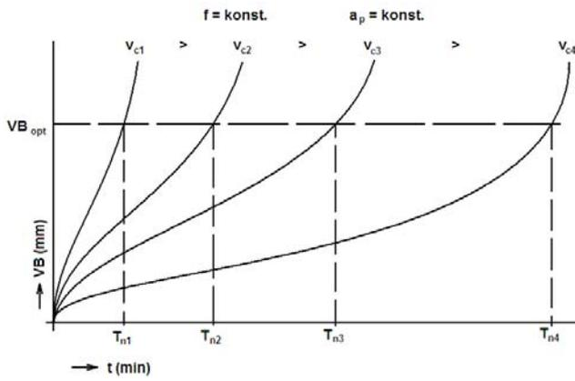
Fig. 1 Blunt curves at variable cutting speed,  $f = \text{konst.}$ ,
