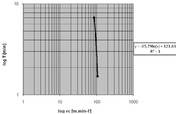
Fig. 8 Logarithmic dependence of durability on the cutting speed for ceramic
