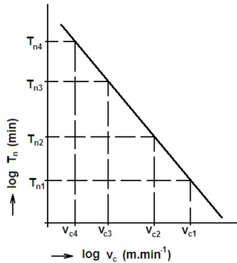
Fig. 3 Dependence – tool-life on cutting speed [1]
