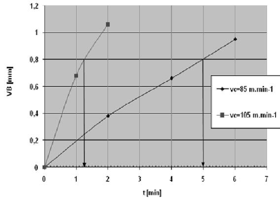
Fig. 4 Curve blunting – cemented carbide
