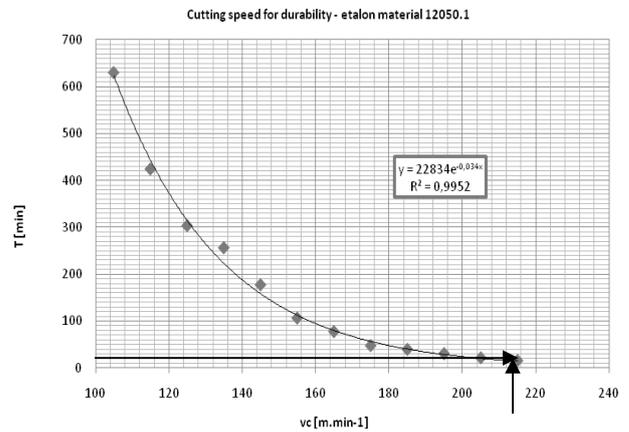
Fig. 4 Determination of tool-life (based on the criterion of wear) for etalon material
