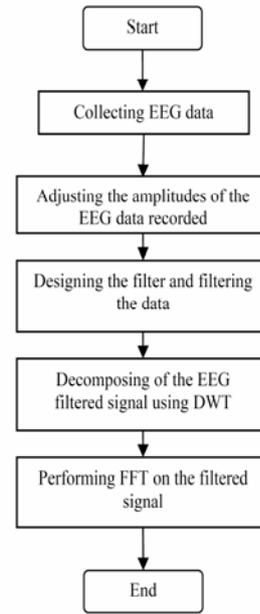
Fig. 6 Flow chart of EEG waves classification procedure.
