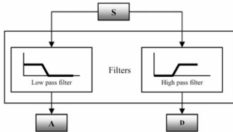
Fig. 4 The filtering process of the DWT
