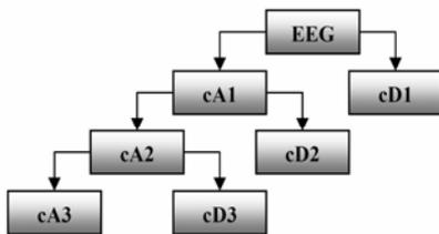
Fig. 5 Sub-band coding algorithm of the DWT
