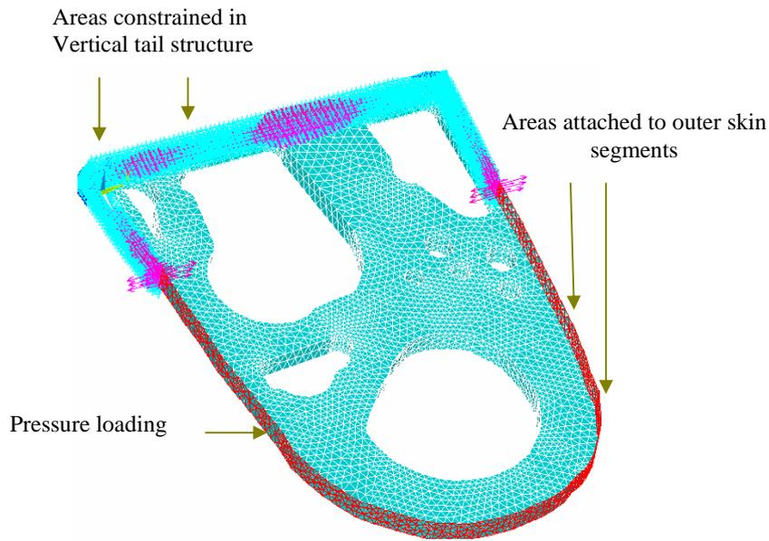
Fig. 7 Loading and constraints on initial optimized model
