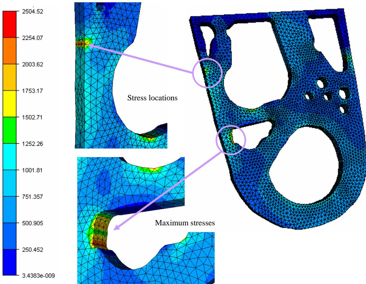
Fig. 6 Structural analysis of the initial optimized configuration
