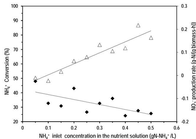
Fig. 4 Ammonium conversion (◇) and specific nitrate production rate (△) as a function of the NH<sub>4</sub><sup>+</sup> inlet concentration in the nutrient solution
