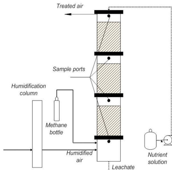
Fig. 1 Biofilter set up for the biofiltration of CH<sub>4</sub>
