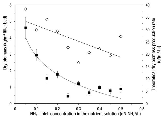
Fig. 3 Dry biomass content (◇) and theoretical dry biomass production rate (■) as a function of the NH<sub>4</sub><sup>+</sup> inlet concentration in the nutrient solution
