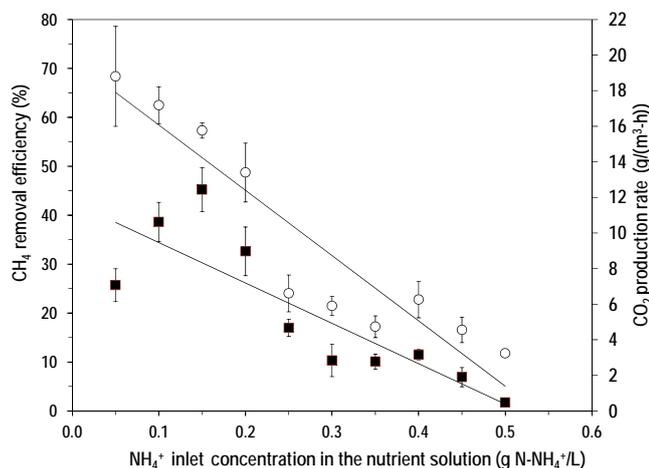
Fig. 2 CO<sub>2</sub> production rate (■) and CH<sub>4</sub> removal efficiency (○) as a function of the NH<sub>4</sub><sup>+</sup> inlet concentration in the nutrient solution
