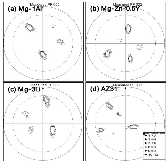
Fig. 4 (0002) pole figures measured on the single crystals of Mg-1Al (a), Mg-Zn-0.5Y (b), Mg-3Li (c) and AZ31 (d) alloys
