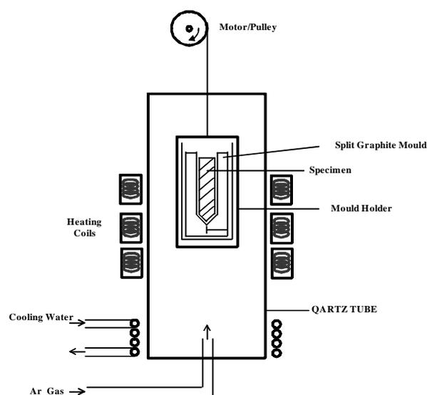
Fig. 1 Schematically illustrated apparatus for single crystal growth
