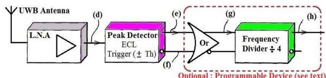
Fig. 5 UWB receiver based on ECL for monocycle pulses
