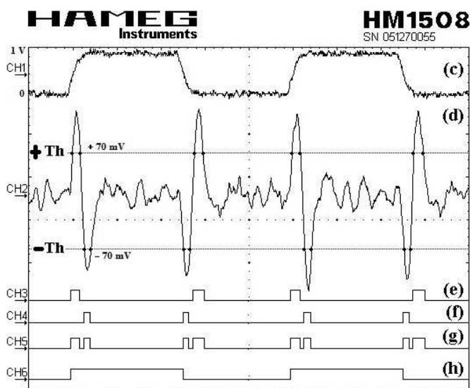
Fig. 6 Detection process
