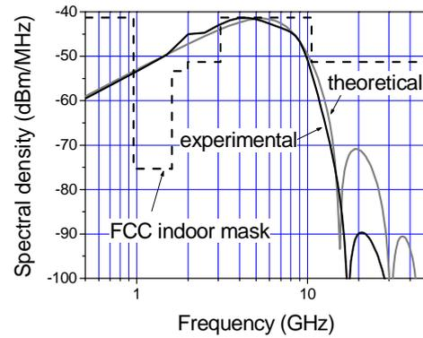
Fig. 3 PSD of the pulse
