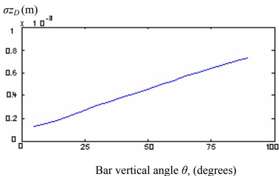
Fig. 5 Standard error of the coordinates  $\sigma_{z_D}$
