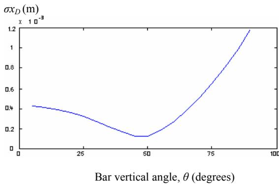
Fig. 3 Standard error of the coordinates  $\sigma_{x_D}$
