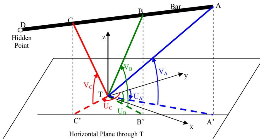
Fig. 1 Geometry of the hidden-point bar method
