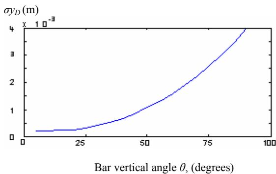
Fig. 4 Standard error of the coordinates  $\sigma_{y_D}$
