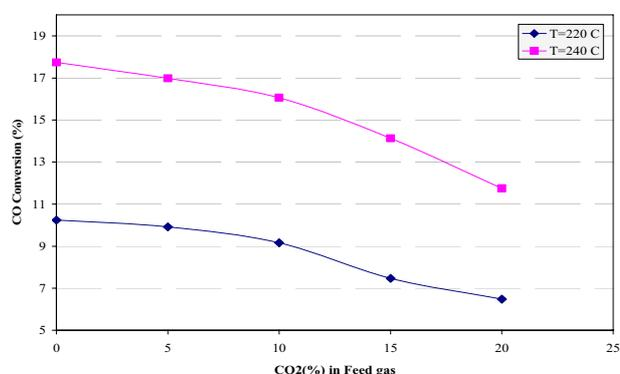
Fig. 9 the effect of CO<sub>2</sub> on CO conversion at 220°C and 240°C
