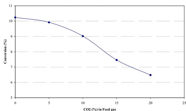
Fig. 7 effect of CO<sub>2</sub> on CO conversion at 220°C
