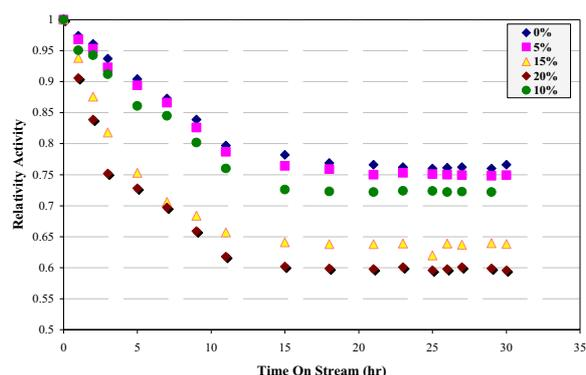
Fig.11 the effect of CO<sub>2</sub> on catalyst deactivation
