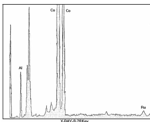
Fig.1 the XRF pattern of Co-Ru/Al<sub>2</sub>O<sub>3</sub>
