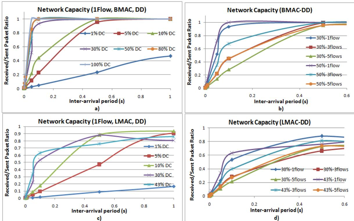
Figure 2: Successful Transmission Measurements Excluding Routing Protocol Overhead
