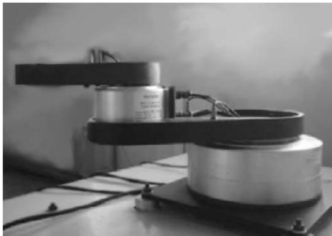
Fig. 1 Two Joint SCARA Type Robot
