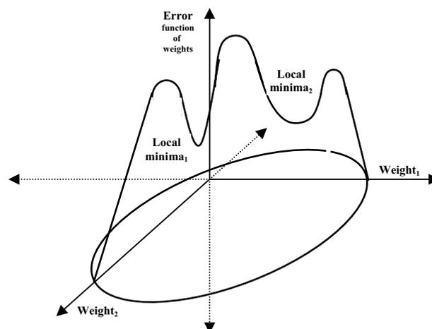
Fig. 6. Valleys in error function cause back propagation algorithm trapped at local minima
