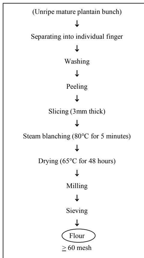
Fig. 1 Flow diagram of preparation of plantain flour
