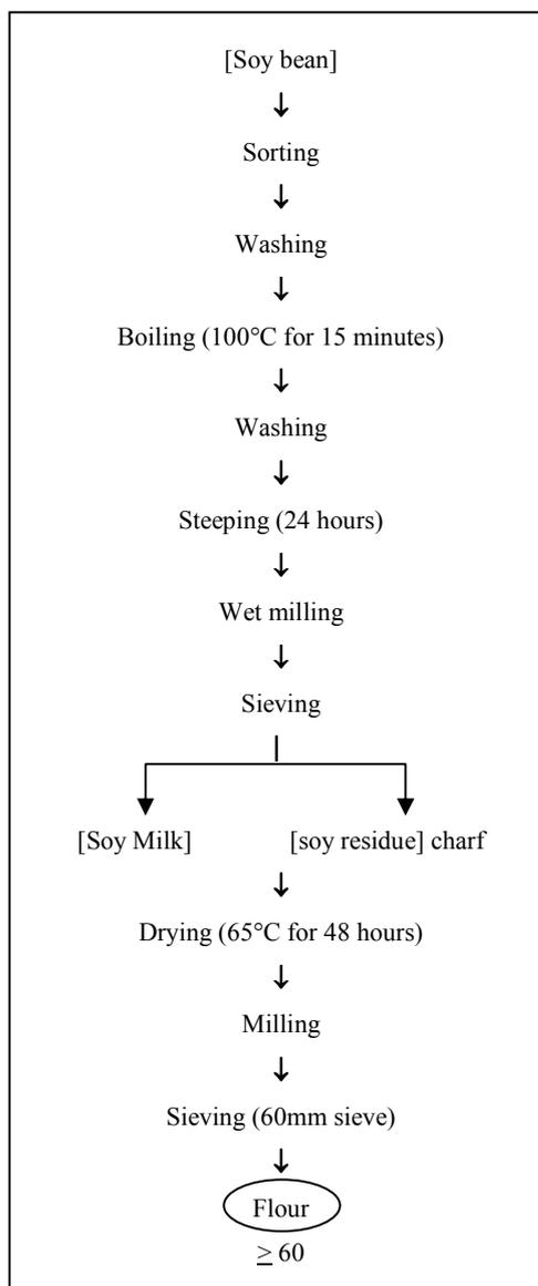
Fig. 2 Flow diagram of preparation of soy residue flour
