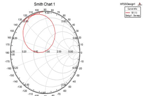
Fig. 4 Smith chart of bowtie antenna at 2.5 GHz
