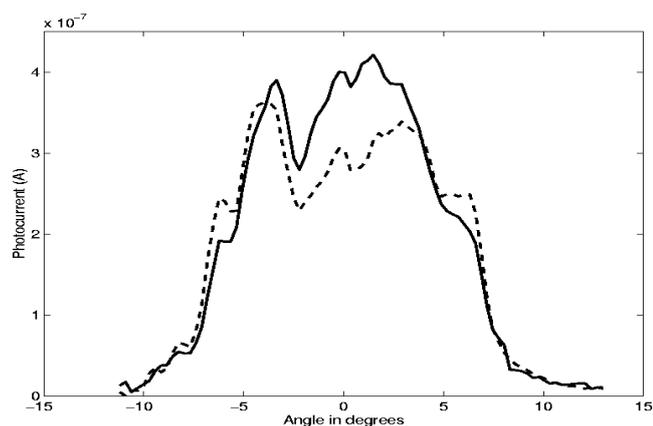
Fig. 4 Beam divergence angle distribution at 1.25 Gbps for alternating ones and zeros pattern (solid), alternating sixteen ones and sixteen zeros (dashed)
