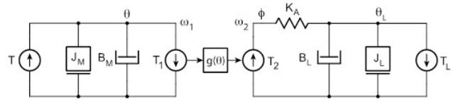
Fig. 3 Flexible coupling – equivalent mechanical circuit
