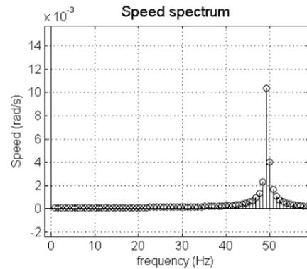
Fig. 8 Speed frequency spectrum with zoom in the fault frequency
