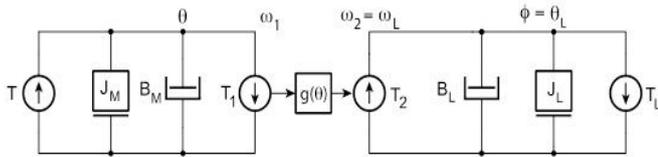
Fig. 2 Rigid coupling – equivalent mechanical circuit
