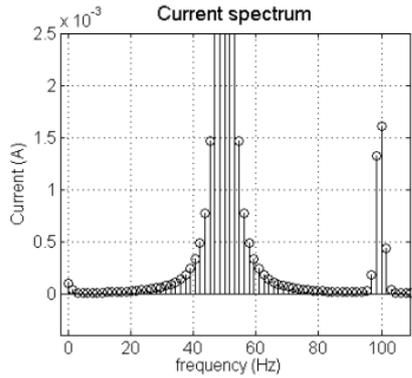
Fig. 10 Current frequency spectrum with zoom in the fault frequency plus supply frequency
