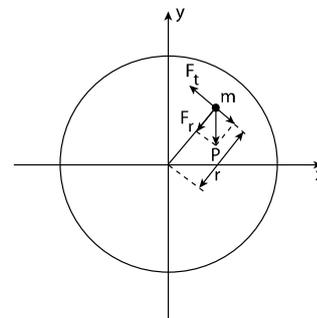
Fig. 4 Model for static unbalance
