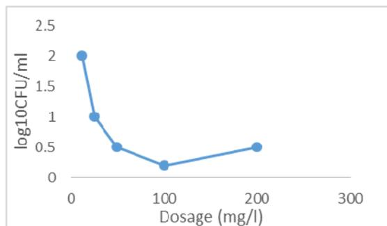
Fig. 1 Effect of dosage on the disinfection process
