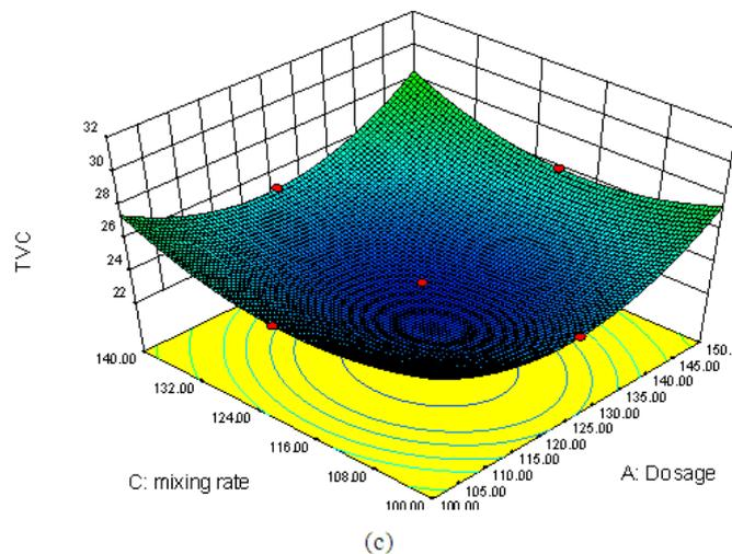
Fig. 4 The 3D curves of combined effects of dosage, contact time and mixing rate of the disinfection process conditions on *E. coli* bacteria strain: (a) contact time and mixing rate (b) contact time and dosage (c) Dosage and mixing rate
