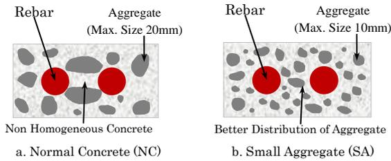
Fig. 11 Coarse Aggregate Distribution at Congested Area
