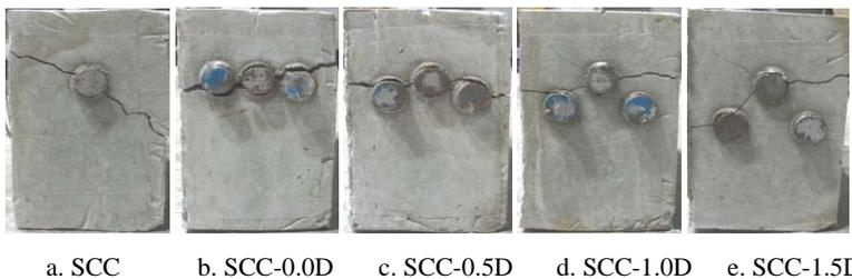
Fig. 14 Fracture Pattern of SCC
