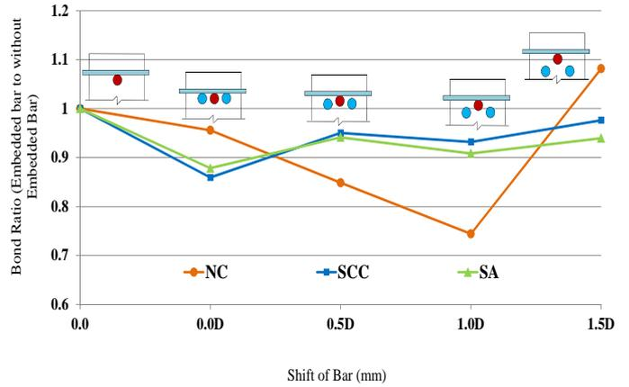
Fig. 12 Relationship between Bond Ratio-Shift of Bar
