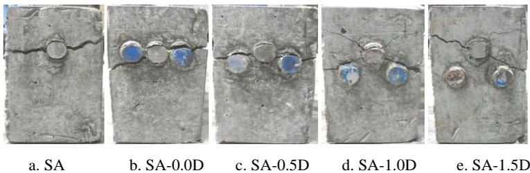
Fig. 15 Fracture Pattern of SA
