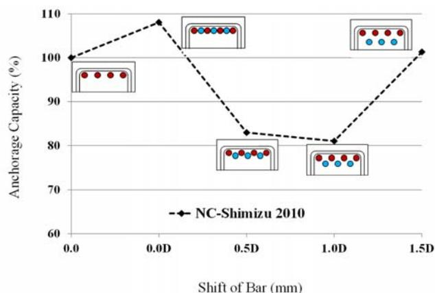
Fig. 3 Relationship between Anchorage Capacity-Shift of Bar
