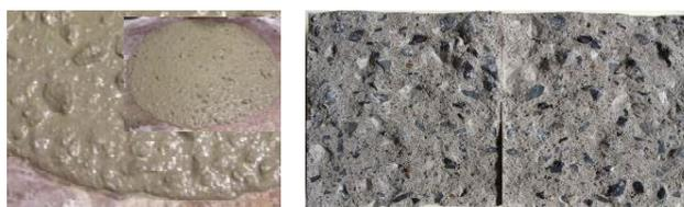
Fig. 5 SCC Behavior showing no sign of Segregation
