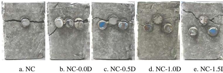
Fig. 13 Fracture Pattern of NC
