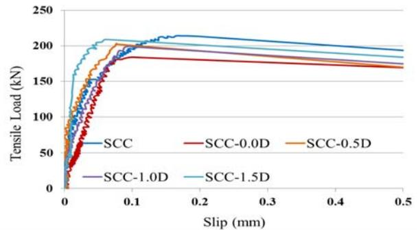
Fig. 9 Load – Slip Relationship for SCC
