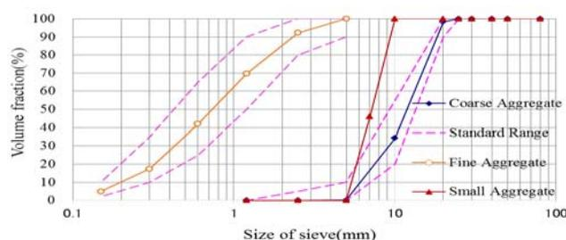
Fig. 4 Gradation of Aggregate for NC and SCC
