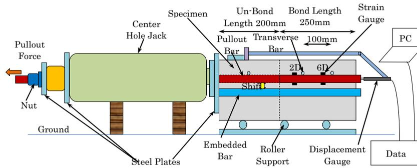
Fig. 7 Experimental setup and Specimen Detail
