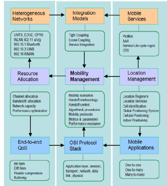
Fig. 4 System Architecture for Vertical Mobility
